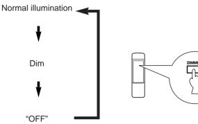
While the display illumination is off, the AUTO DISPLAY OFF indicator on the front panel is illuminated.
