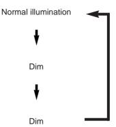
(The AUTO DISPLAY OFF indicator lights up. In this mode, if a disc is played, the display illumination will be turned off.)
